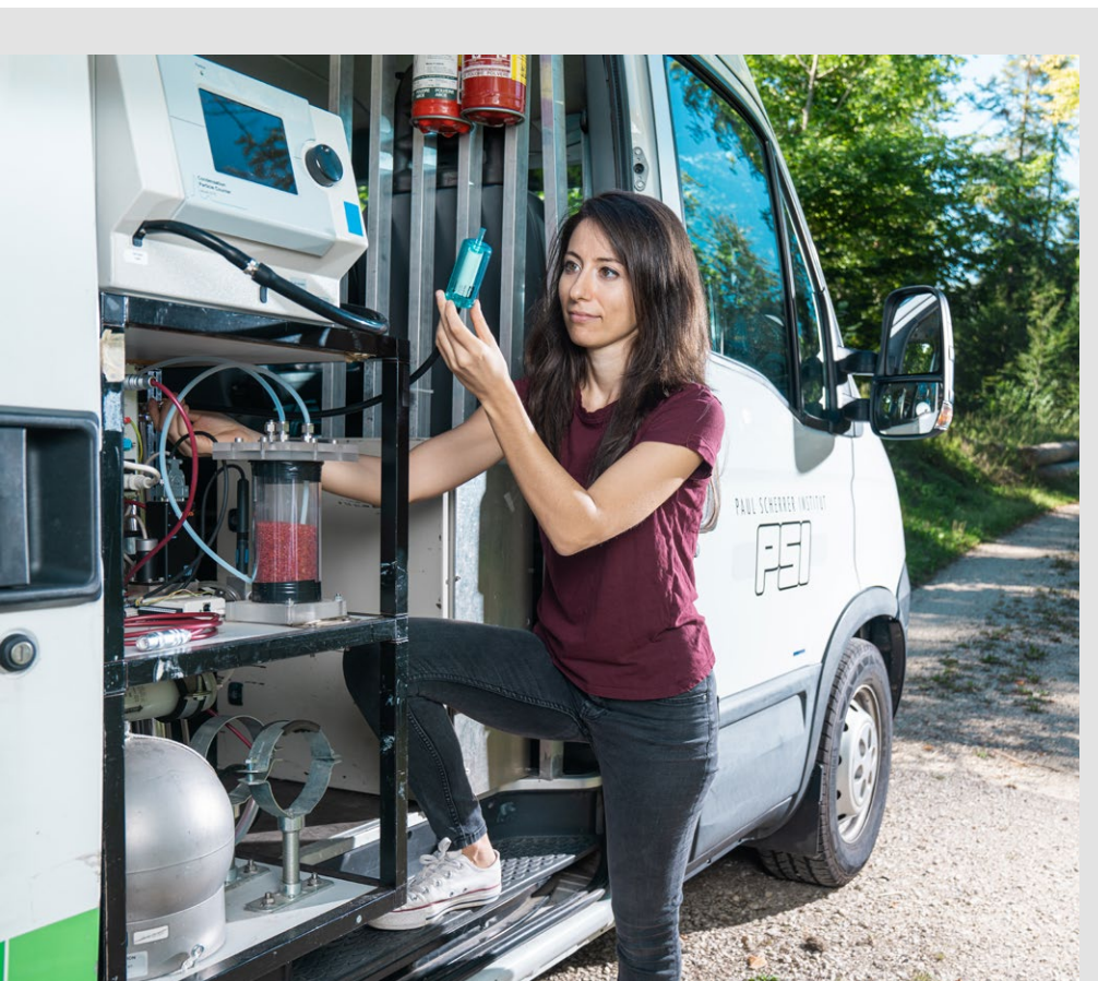
PSI's smogmobile. Various devices, including an apparatus that draws air through the pores of a filter, can be installed in it. Researchers can then analyse the accumulated material.
